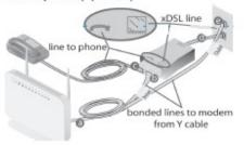
voice service is connected. A technician may need to identify this for you. In North America the inner pair is normally red and green.
