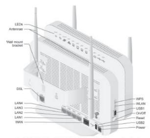
Verify that the POWER LED is solid red or green indicating local power is on and voltage is good. See the user guide for a complete description of the LEDs
